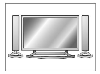
For proper ventilation, allow a clearance of 4" on each side and the top, 2.36" on the bottom, and 2" from the wall. Detailed installation instructions are included in the optional Desktop Stand Installation and Setup Guide, see your dealer.
